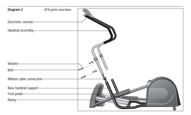
CAUTION: Do not install the handrail assembly until you move the EFX to its final location. Ask for assistance to move the unit.
